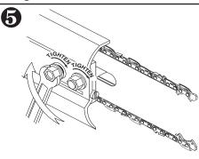
Make sure chain moves freely around guide bar then tighten both nuts.
